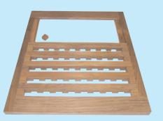
8. Now lay the castles in the outer frame, placing a 7/8" flat spacer in between. If necessary, trim each spacer with a sharp chisel to end up with even spacing. Make sure the grain of the spacer blocks run parallel with the runners (see right).
