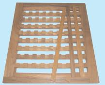
11. Next day remove the clamps. Turn upside down and remove any surplus glue in corners etc with a sharp chisel. Now cut the flat infills to length and glue, making sure all mating surfaces are wet with epoxy. Do the same with the infill blocks. Now leave over night.
