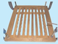
10. Glue the outer frame making sure you wet all mating surfaces with epoxy. Gclamp the 4 corners as shown. Now glue the castles and blocks in position. Place a flat infill underneath (making sure no epoxy comes into contact it) to ensure the castle sections line up. Now leave over night to dry.
