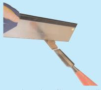
7. To cut the castle profile, cut vertically with a tenon saw and lightly tap a sharp chisel horizontally to remove.
