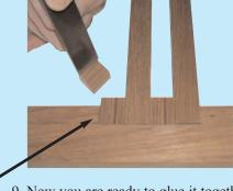
9. Now you are ready to glue it together. The epoxy should be mixed 5 parts Epxoy Resin to 1 part Hardener (using the marked stick provided) in a suitable container.
