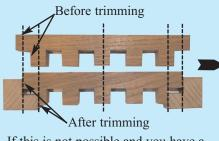
5. If this is not possible and you have a full depth castle falling on the outer frame, centralise the castle section and cut both sides (as shown), making sure they are exactly the same.
